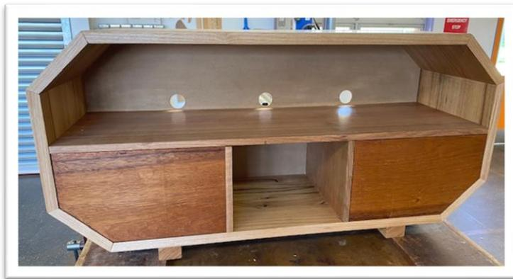
Samuel's HSC Industrial Technology major project, he designed and built a television cabinet out of Mountain Ash. He started his project at the start of Term 4 last year and finished it around the end of August 2021. Most of that time was spent joining timbers together to create the desired width of timber for the carcass of his cabinet. The design is unique, and the drawer fronts had to be cut to fit and they operate on push to open drawer runners, so no need for handles.
