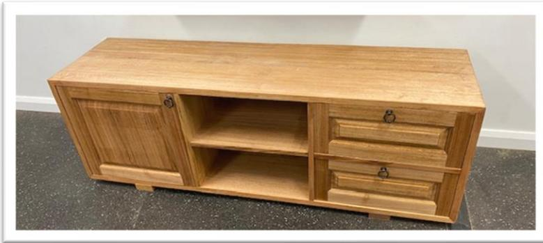
Leith's HSC Industrial Technology major project, he designed and built a television cabinet out of Mountain Ash. He started this project around the start of the year and finished it around the end of August 2021. Most of that time was spent joining timbers together to make the desired width of timber for the carcass of his cabinet. Door and drawer fronts have been profile cut for an added feature.
